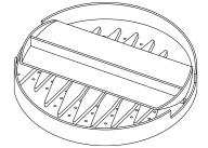
Mechanical distribution of the wastewater on the entire surface of the BIOROCK media.
