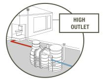
Our high-level discharge is equipped with a reliable, high quality, pump kit. This kit is delivered pre-assembled for ease and speed of installation. Intermittent operation by float switch.
